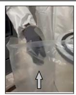
Remove the displacer from the filter cartridge.
